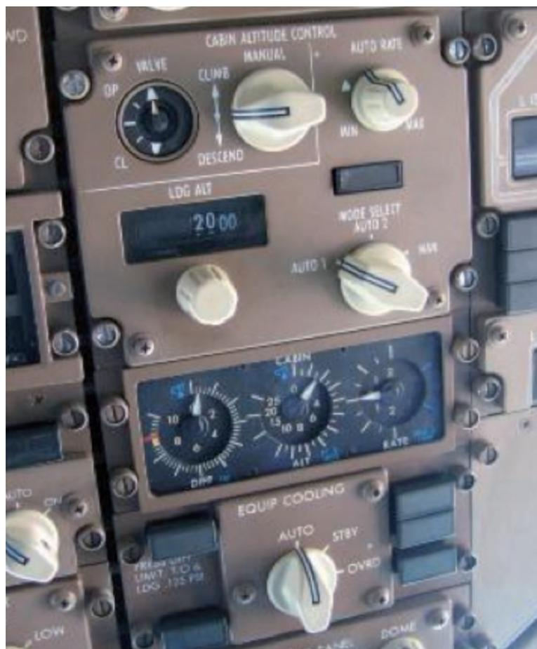
**Figure 12. Cabin altitude control panel**
