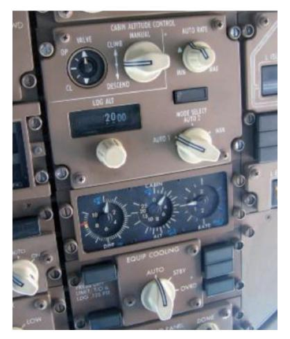
Figure 12. Cabin altitude control panel
