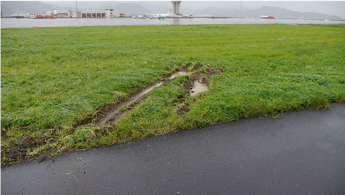
Figure 3. Tracks left by the nose wheel on the ground
