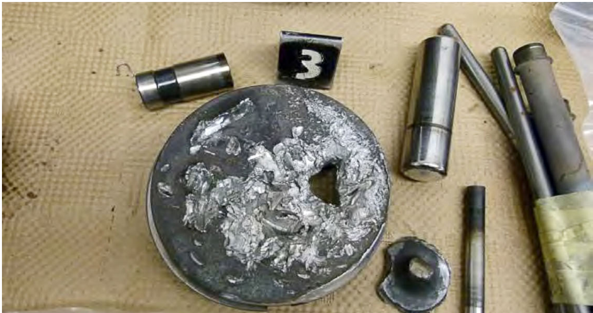
Figure 5. Piston, valve and other components of the no. 3 cylinder
