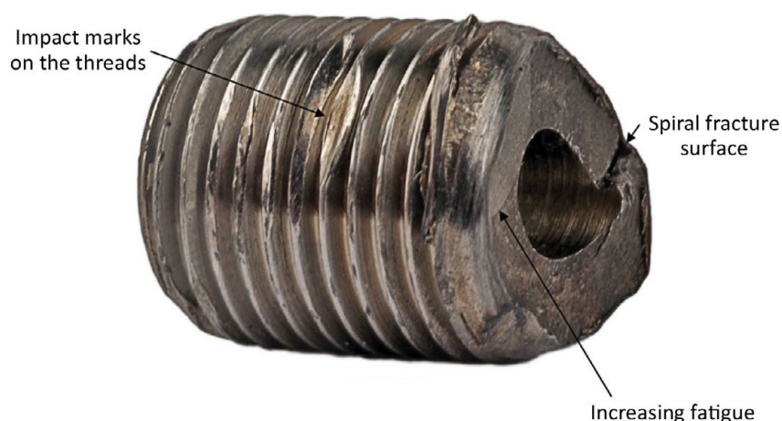
Figure 10. Damage on the threaded end of the PT shaft
