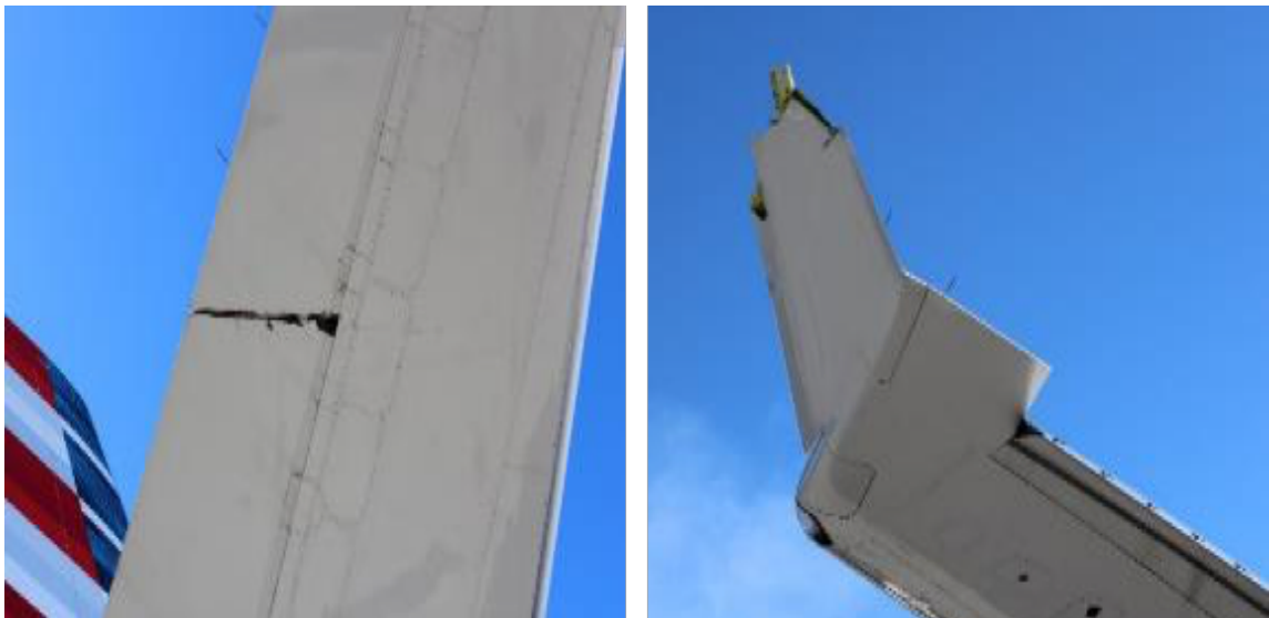
Figure 3. Photograph of the cut in the right elevator of aircraft N758AN (left) and of the left wingtip of aircraft EC-LZX (right)
