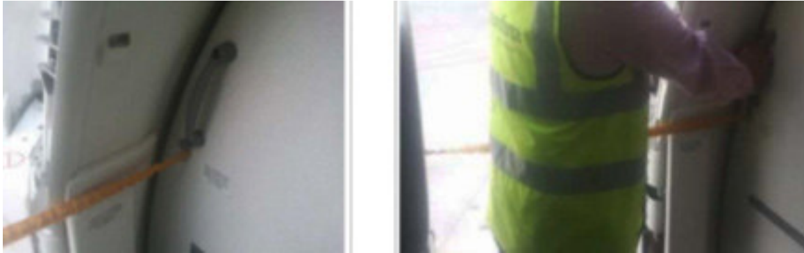
Figure 1. Close-up of the handle and safety strap (left) and reconstruction of the AMT's position (right)
