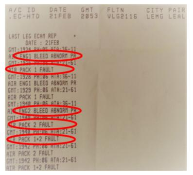
Figure 1. Post-flight report showing warnings on the ECAM display
