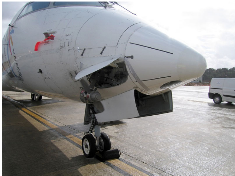
Figure 1. Aircraft after landing with the ADG deployed
