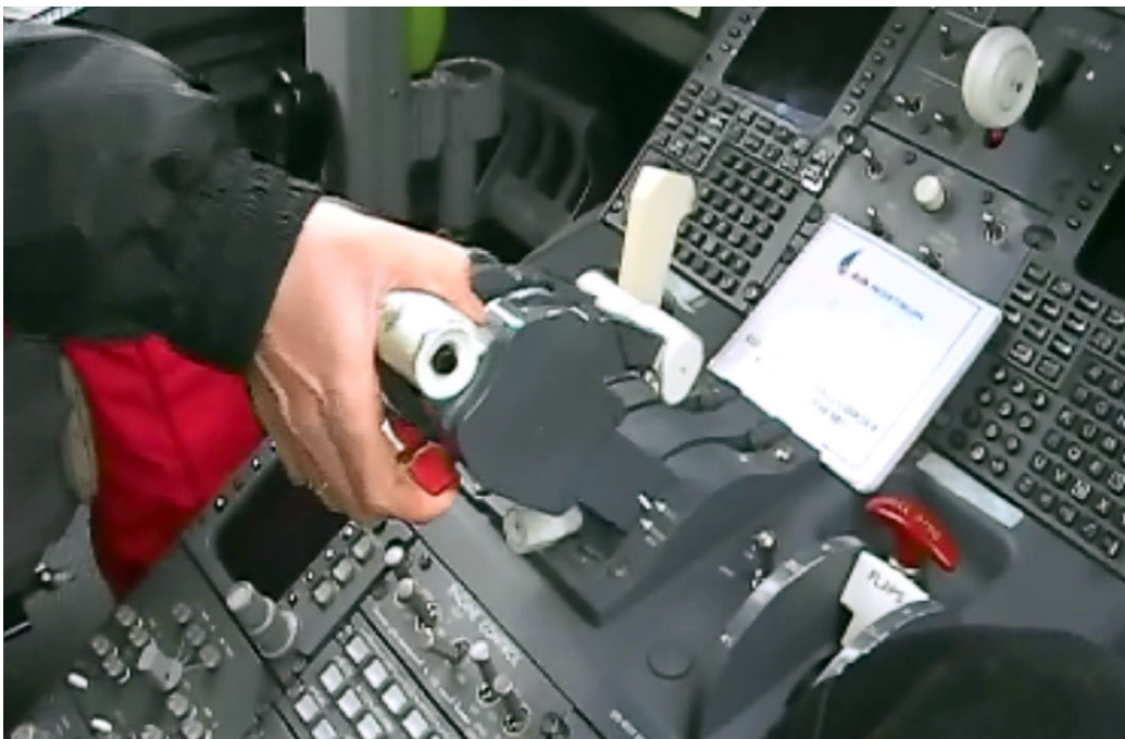
Figure 5. Positioning the lever from IDLE to SHUT OFF
