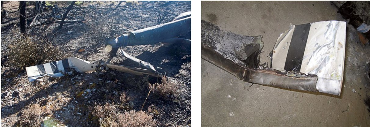
Figure 24. Tail rotor debris
