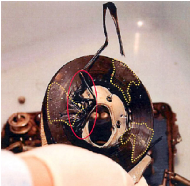
Figure 12. Condition of the magnetic tape
