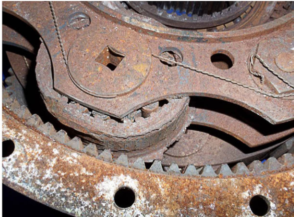
Figure 5.3. Close-up of gears on lower planetary gear
