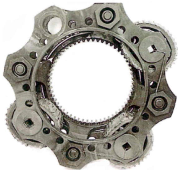
Figure 22. Condition of the lower planetary gear in the second case
