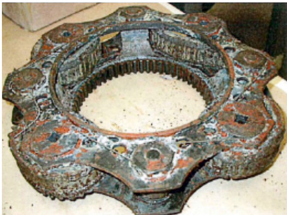
Figure 21. Condition of the lower planetary gear in the first case
