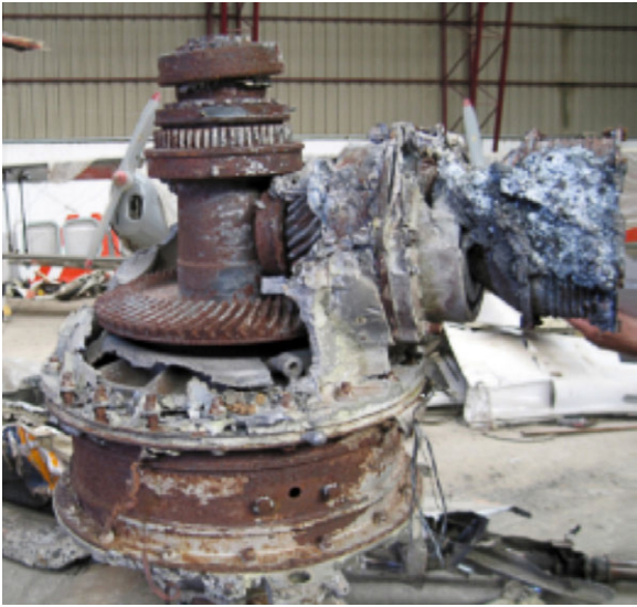
Figure 5.1. External condition of MGB
