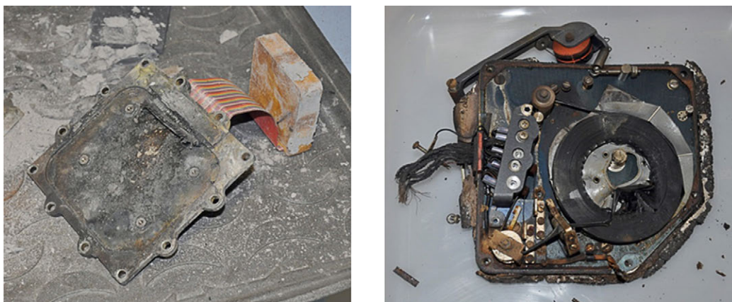
Figure 10. Condition of the flight recorders after recovery
