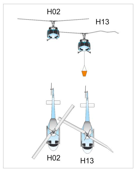
Figure 6. Position of the two aircraft just before the impact of the second blade
