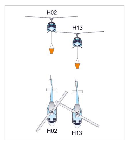
Figure 5. Position of both aircraft just before the impact of the first blade
