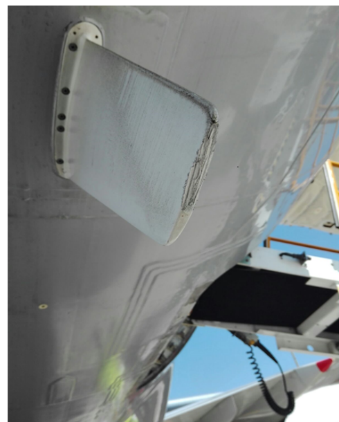
Fig. 2. Details: VHF antenna and sewage drainage probe damages.
