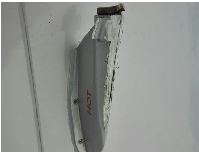
Fig. 2. Details: VHF antenna and sewage drainage probe damages.
