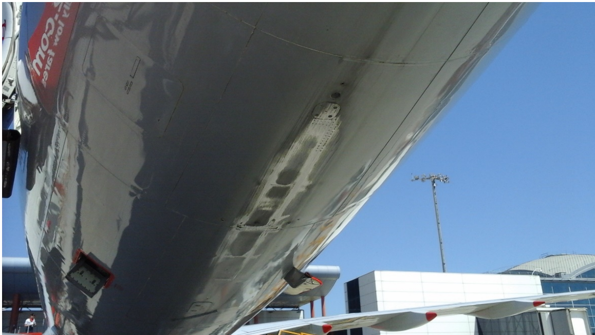
Fig. 1. Damage to the rear underside of the fuselage.
