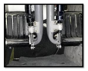
Figure 16: Master actuator pistons of the co-pilot's brake pedal.
