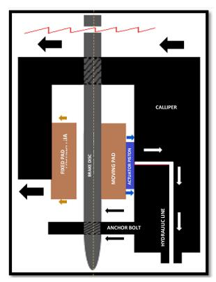
Figure 25: Operation of the brake (4).
