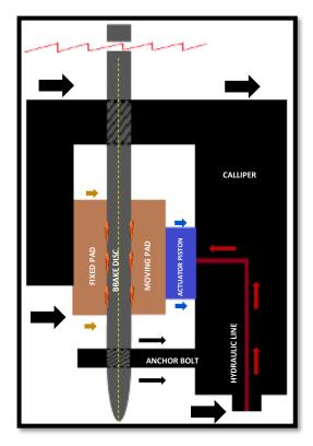
Figure 24: Operation of the brake (3).
