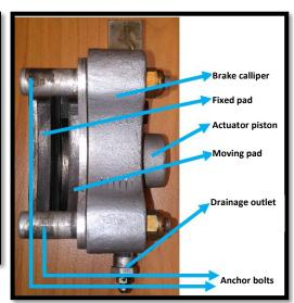
Figure 20: Brake (plan view).
