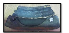
Figure 13: Fixed pad after the accident.
