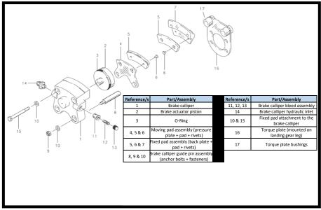
Figure 3: Diagram of the aircraft's brake.
