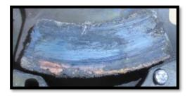
Figure 12: Moving pad after the accident.
