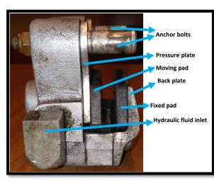
Figure 19: Brake (side view).
