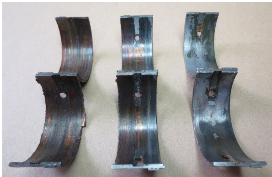
Figure 10. Photograph of the crankshaft bearings (left front support, central centre support and right rear support)
