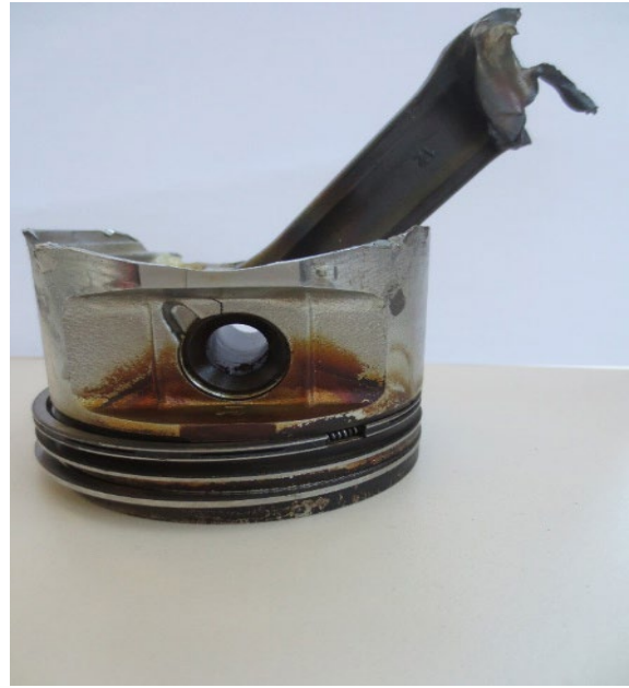
Figure 9. Photograph of cylinder no.1's crankpin, with one part of the connecting rod (left) and piston no.1 with the other part of the connecting rod (right)
