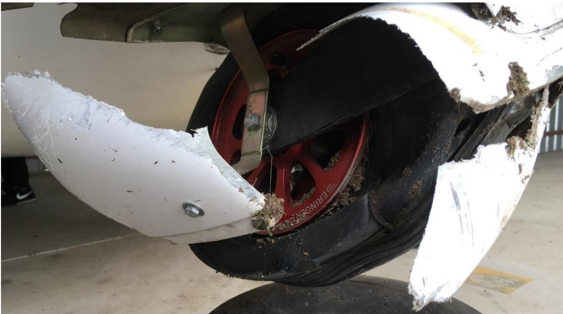
Figures 8 (previous page, bottom), 9 (this page, top) and 10 (this page, bottom): damage to the nose leg
