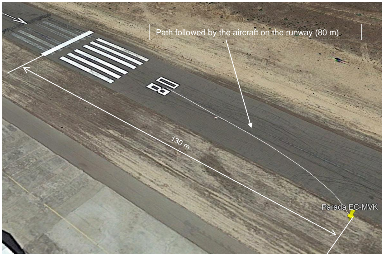
Figure 3: Approximate path followed by the aircraft as it dragged along the runway after the second bounce.
