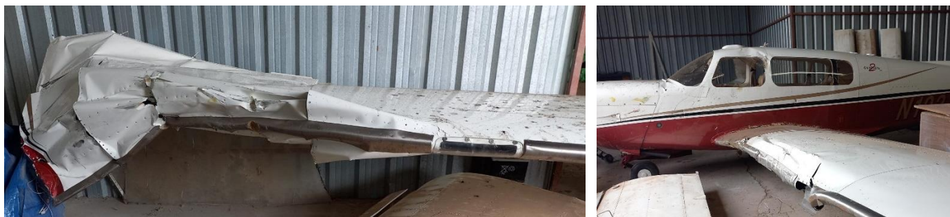
Figure 6. Damage to the wings
