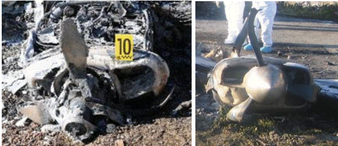
Illustration 6: Photographs of the right engine (left) and left engine (right) propeller blades
