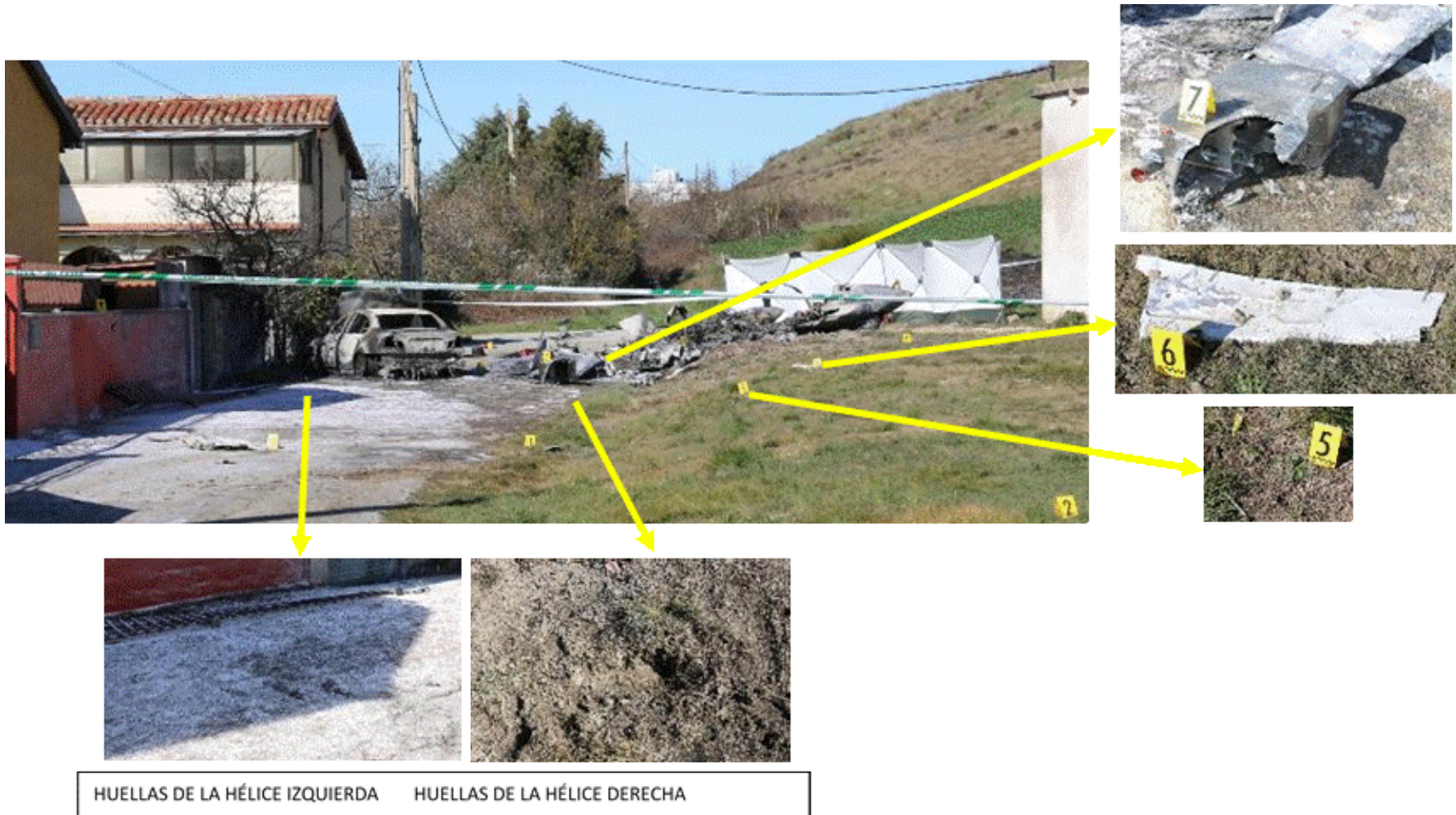
Illustration 5: close-up of the propeller marks and, to the right, the right elevator (number 6)
