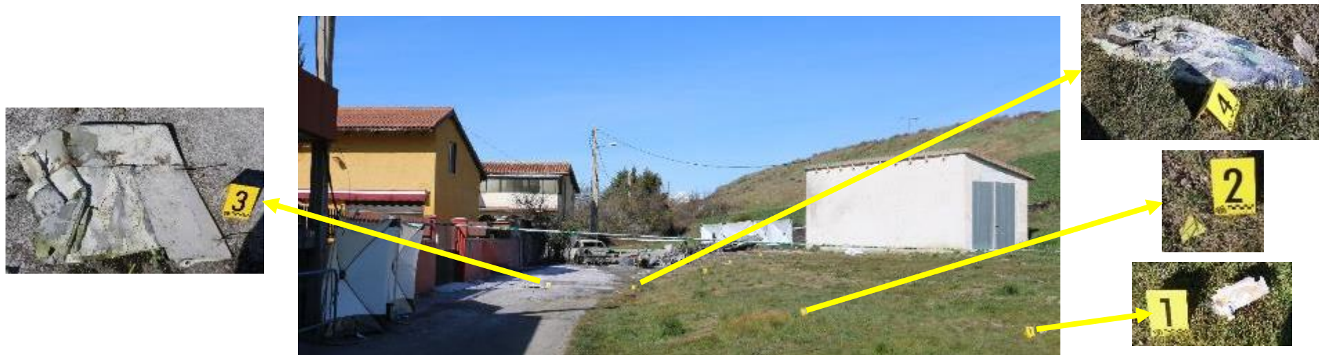
Illustration 4 on the left, the left wingtip (number 3), and on the right, part of the tail cone, number 4
