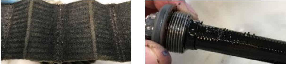
Photograph 17. Presence of particles in the interior of the oil filters
