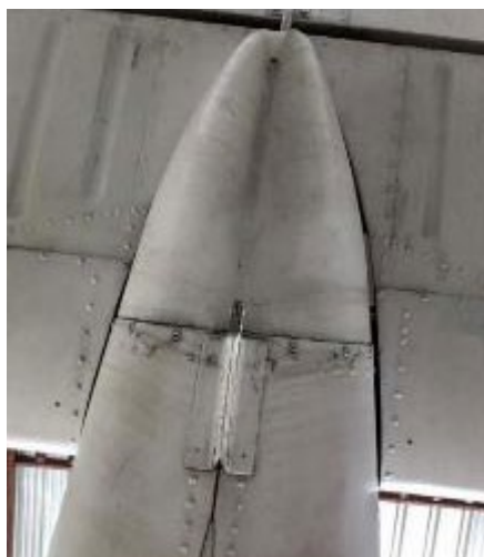
Photograph 13. Damaged tie-down ring
