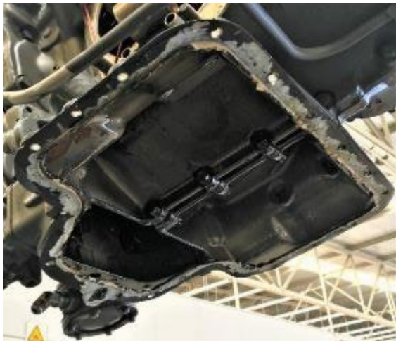
Photograph 29. Sealant on the surfaces of the sump
