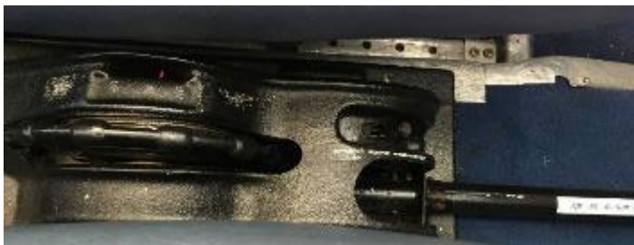
Photograph 15. Automatic landing gear extension system, flap and compensator
