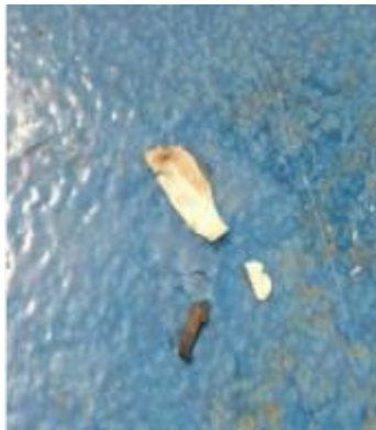
Photograph 26. Particles in the oil in the sump
