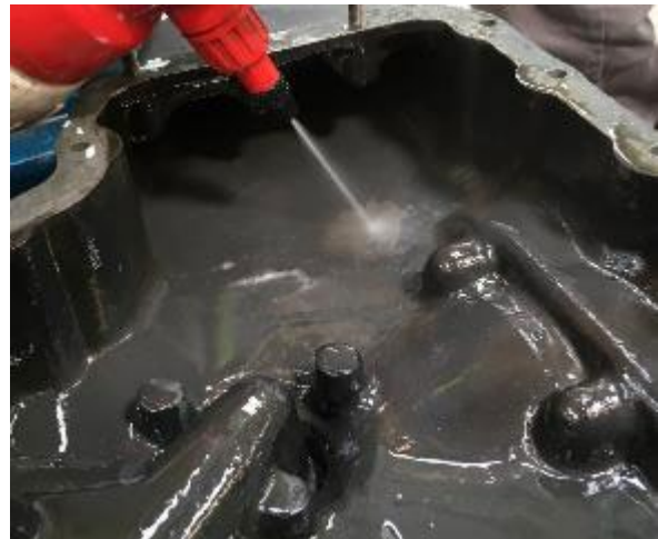
Photograph 30. Sludge and dirt in the sump
