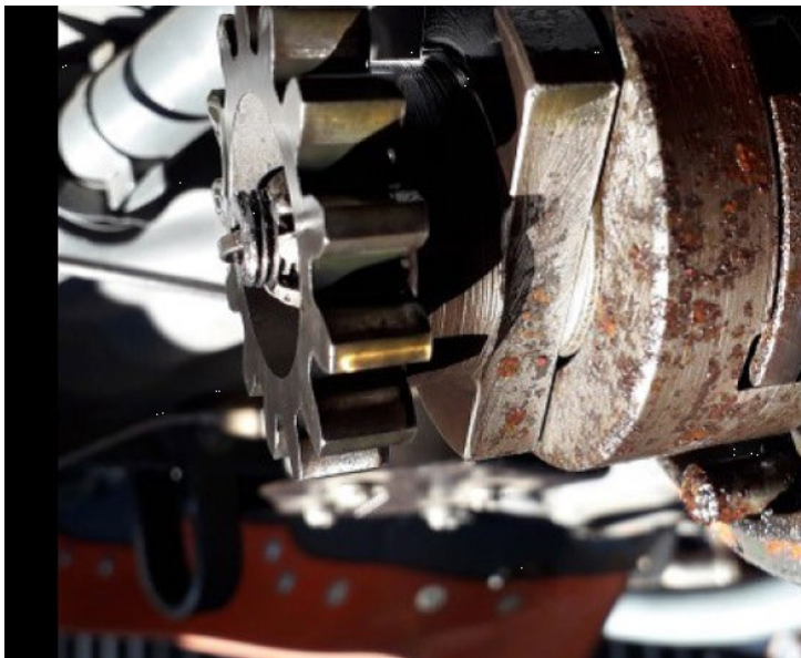
Photograph 18. Presence of corrosion in the left magneto
