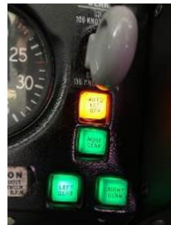
Photograph 3. Landing gear position lights
