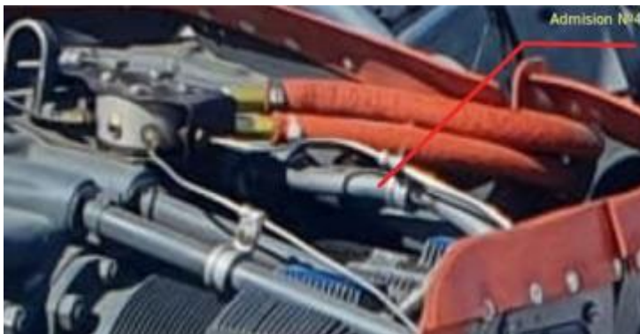
Photograph 20. Cylinder no. 4 intake valve guide
