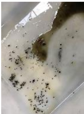
Photograph 26. Particles in the oil in the sump
