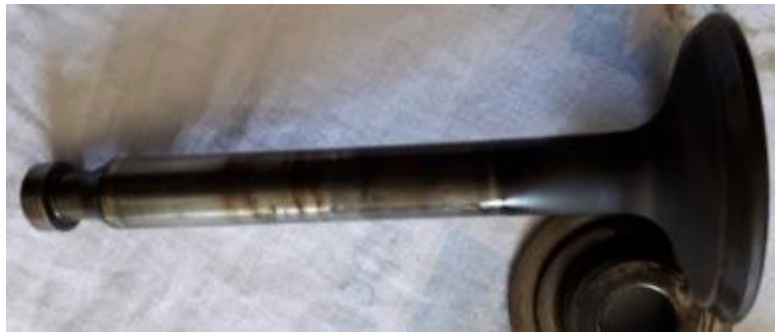
Photograph 24. Cylinder no. 4 exhaust valve
