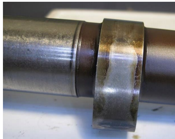
Photograph 36. Cam wear and tear
