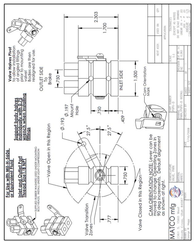
FIG. 12 INSTALLATION OF THE VALVE MATCO PVPV-D(2)
