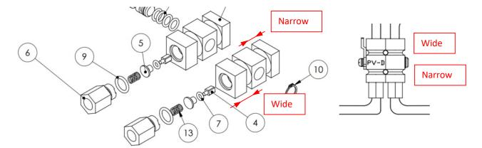
FIG. 9 EXPLODED VIEW AND INSTALLATION OF THE VALVE
