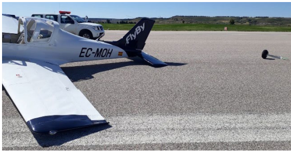
Figure 4. Photographs of the aircraft on the runway and the nut and bolt fragments found on the runway. The left main landing gear had detached, and was on the runway a few metres behind the aircraft (see figure 4).
