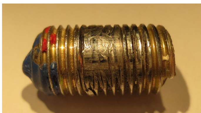
Figure 7. Photograph of the sheared fragment of the inner bolt (MS20006-27)
