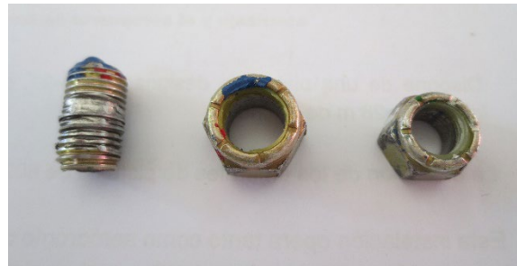
Figure 4. Photographs of the aircraft on the runway and the nut and bolt fragments found on the runway. The left main landing gear had detached, and was on the runway a few metres behind the aircraft (see figure 4).
