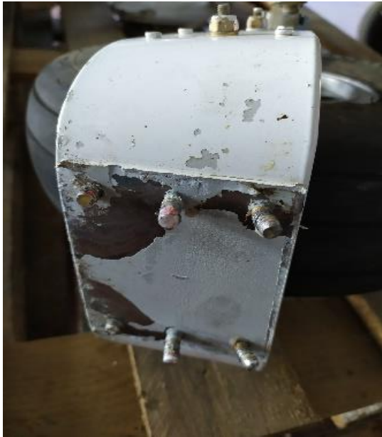
Photograph 15. Area where the fork attaches to the nose gear leg
