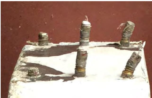
Photograph 11. Connecting plate for the nose gear wheel fork
