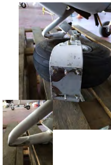
Photograph 7. Damage to the nose landing gear Photograph 8. Detail of the left photo: damage to the side of the nose leg
