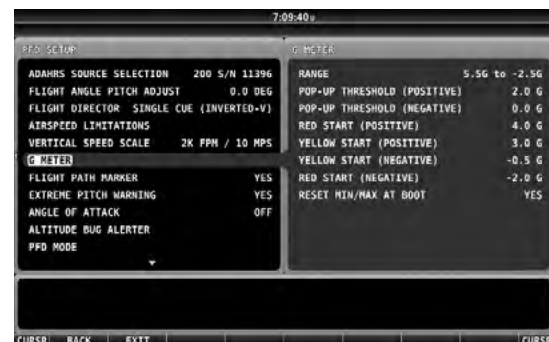
Photograph 3. Set up of the "g" meter in the flight display
