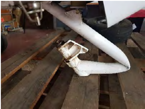
Photograph 12. Buckled nose gear leg
