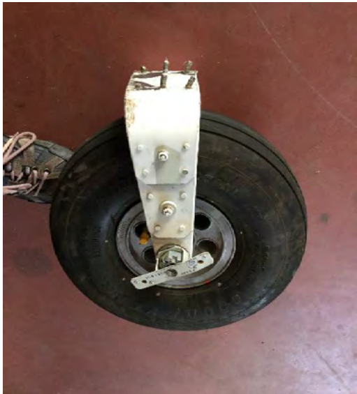
Photograph 14. Nose landing gear wheel and fork
