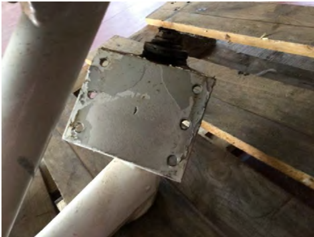
Photograph 11. Connecting plate for the nose gear wheel fork
