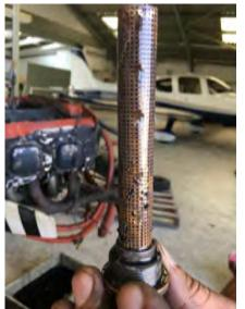
Photograph 19: Oil filter with metallic particles
