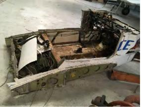
Photograph 9. Aircraft cabin wreckage
