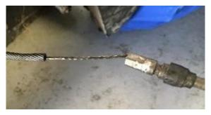
Photograph 14. Detail of the non-crimped mixture controller cable
