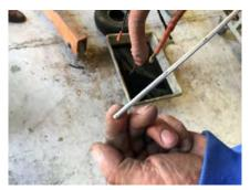
Photograph 17: Oil dipstick and remaining oil in the float bowl
