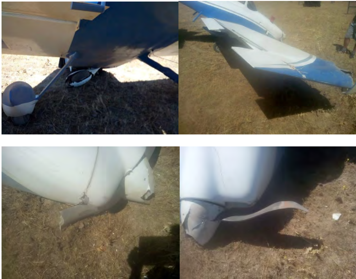
Fig. no. 3 - Detail of the damage to the aircraft
