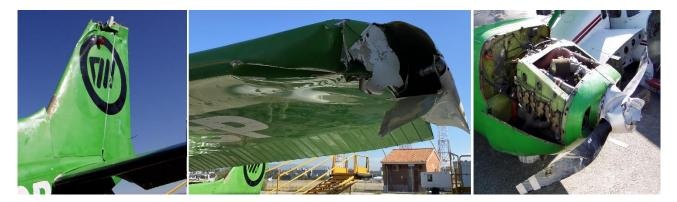
Figure 3. Damage to the aircraft
