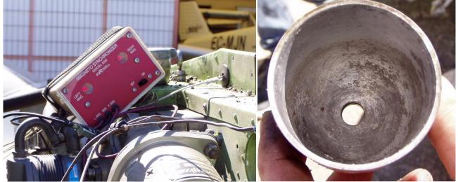
Figure 5. Magnetos check and disassembly of the gascolator filter bowl
