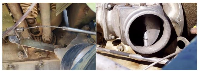
Figure 4. Mixture cable jacket and alternative air valve
