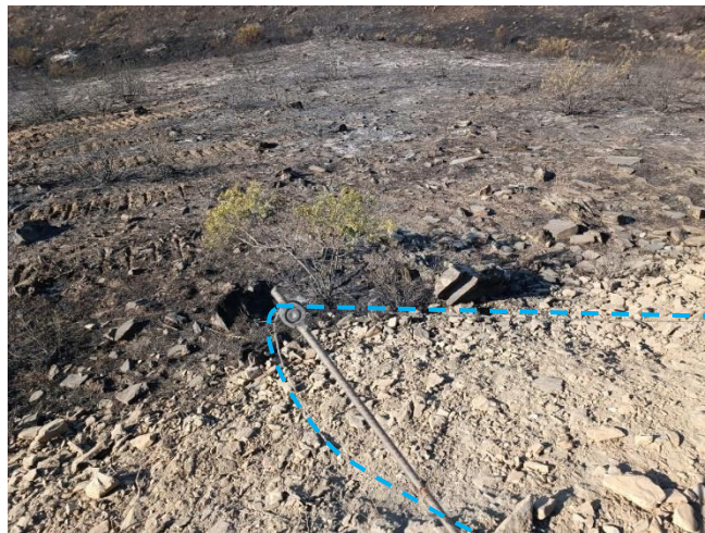
Photograph 8. Electrified fence rod bent after the accident, with the end of the electrified wire
