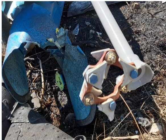
Photograph 13 left. Breakage of tail rotor attachment to tail boom.
