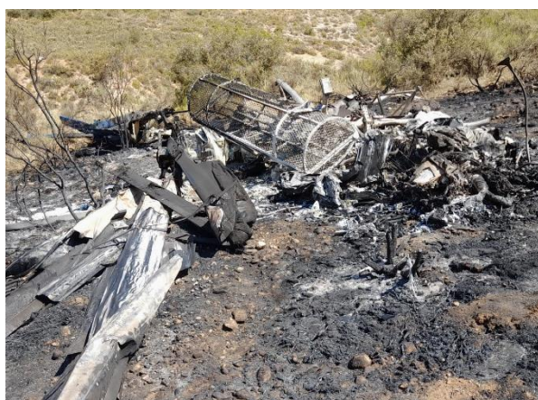
Photograph 9. Melted engine, helibucket carrier and main rotor blades
