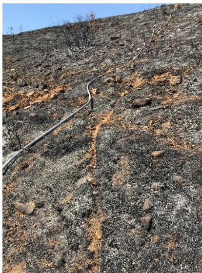
Photograph 20. Severed cable from the southern slope
