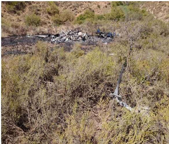
Photograph 11. Tail rotor at the accident site
