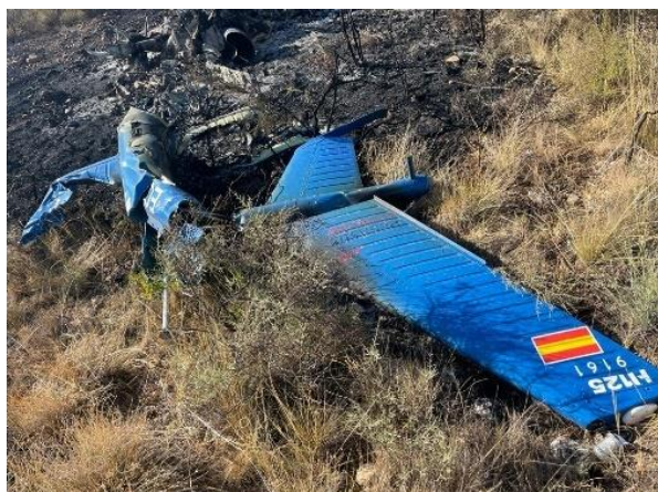
Photograph 7. Empennage and tail boom section
