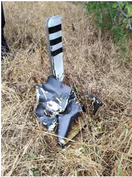
Fig. no. 3 - Detail of the tail rotor.
