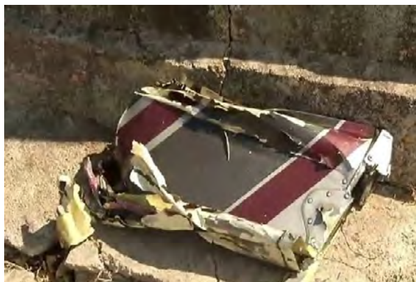
Fig. no. 4 - Helicopter's stabiliser: main body and detached upper part
