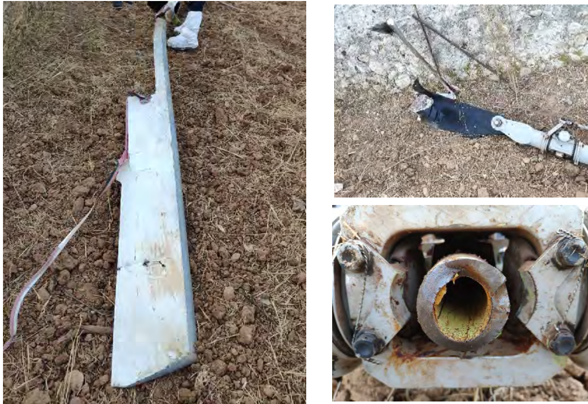
Fig. no. 2 - Detail of the rotor head and damage to parts of the blades.
