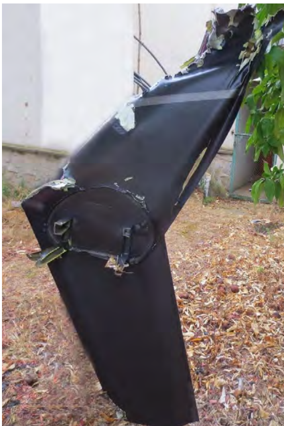
Fig. no. 4 - Helicopter's stabiliser: main body and detached upper part
