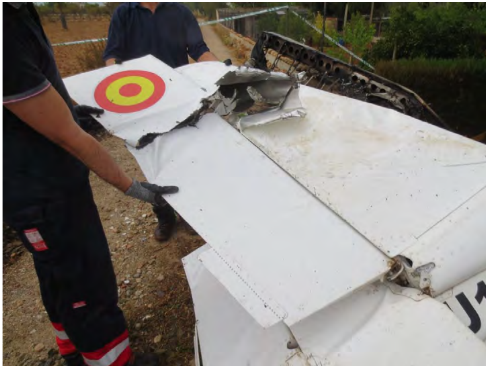
Fig. no. 7 - Detail of the rudder, stabiliser end and the two components together
