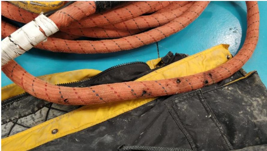
Fig. 5 - Close-up of burn marks on the sling
