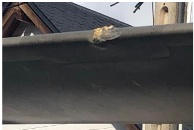
Illustration 14: Detail of the damage to one of the main rotor blades
