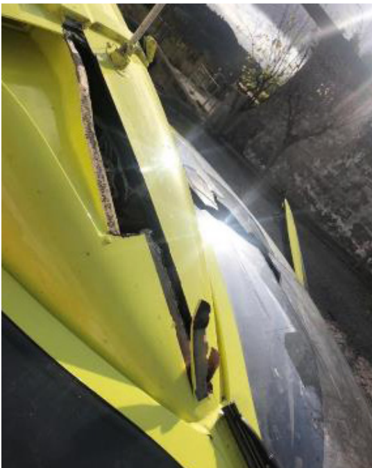
Illustration 13: Detail of the damage to the front window and cable cutter
