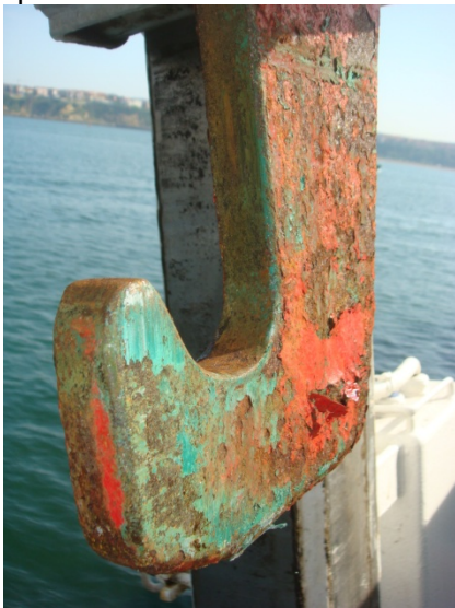
Photo 10: The hooks used on board with blunt end.
