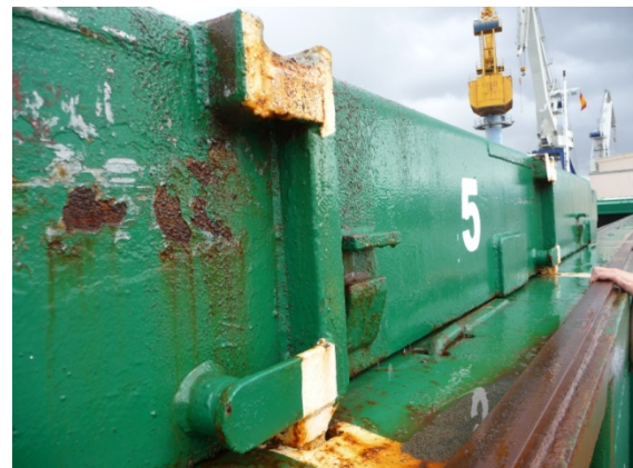
Photo 11: Hatch with two attachment points with rounded profile.
