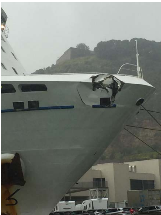
Figura 9. Damage to the starboard forecastle and the weather deck
