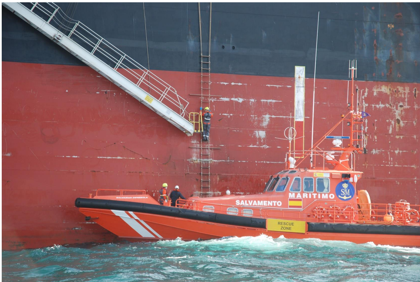
Figura 8. Reconstruction on the BORDEIRA's starboard combination ladder. Height from which the crew member fell. Source: Judicial Police
