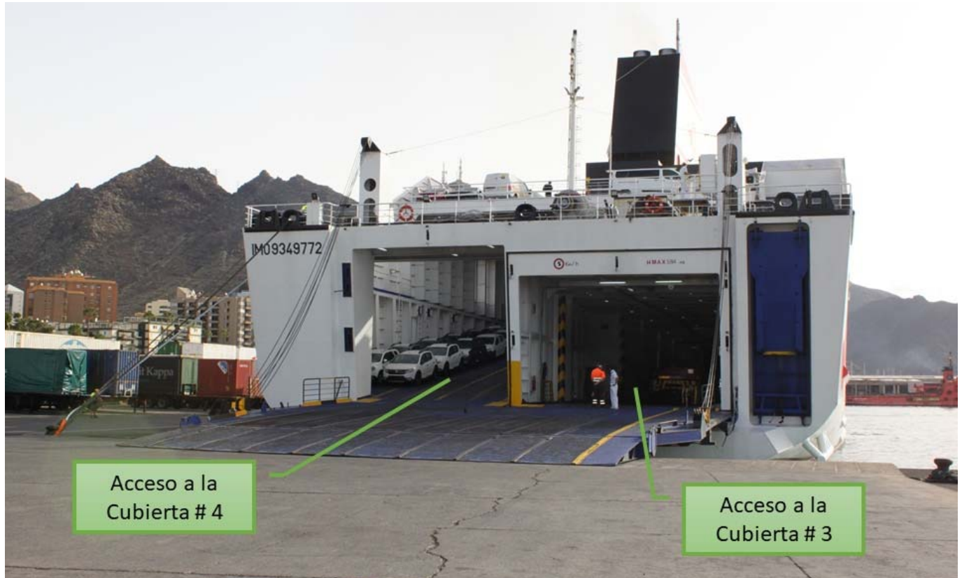
Figure 4. The CIUDAD DE PALMA docked, with stern facing the loading dock for vehicle freight and ramp lowered, at the port of Santa Cruz de Tenerife.
