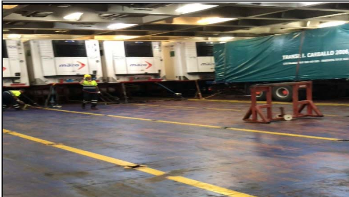
1. The dockers and crew prepare the materials required for stowing and tying down. A trestle is visible in the foreground, and in the background on the left some crew members are preparing the straps.
