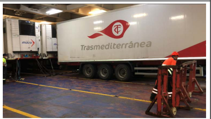
8. The dockers bring trestles over to the area. The crew members move in to tie down the trailer.
