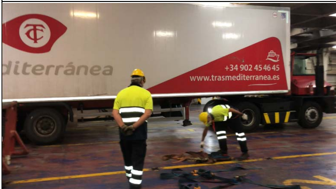
7. Trailer in position. The driver stops the tractor unit. The crew members gather the tying-down material.
