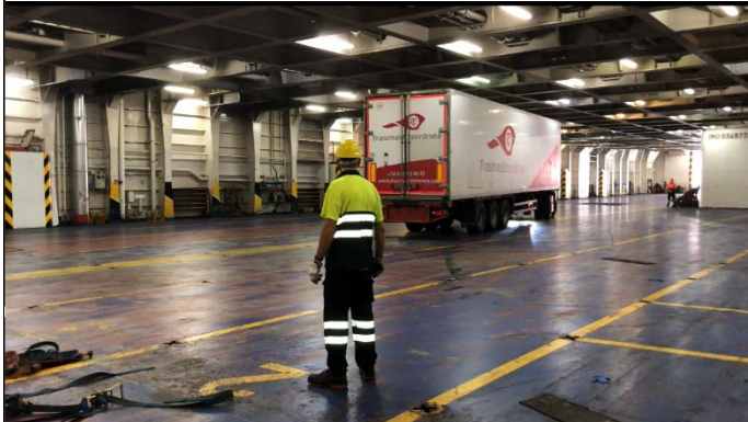
5. The tractor-trailer stops. The driver attempts to position the trailer in the correct row. The unit switches from "towing" to "pushing".
