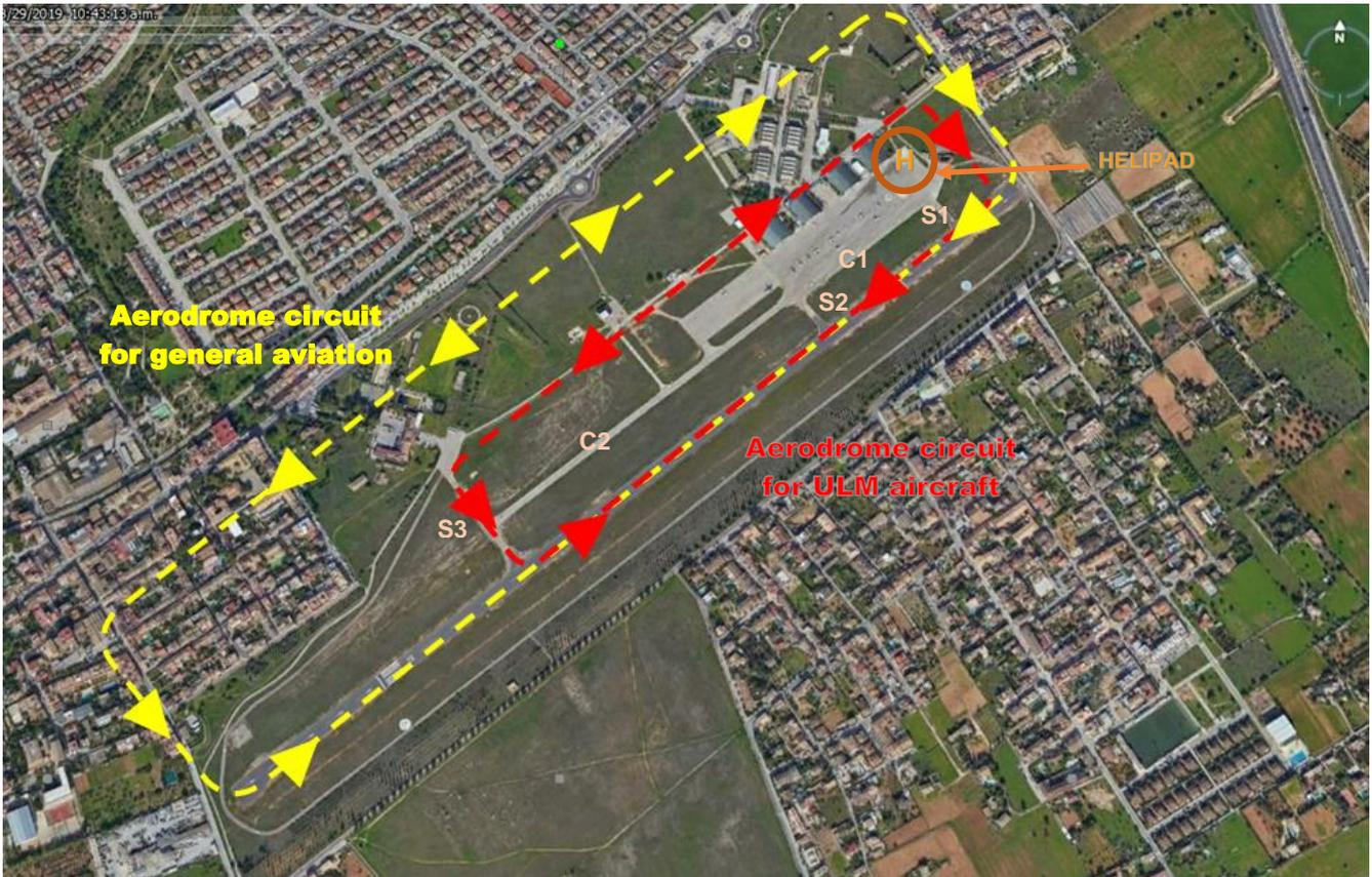
**Figure 5. Aerodrome circuit**
