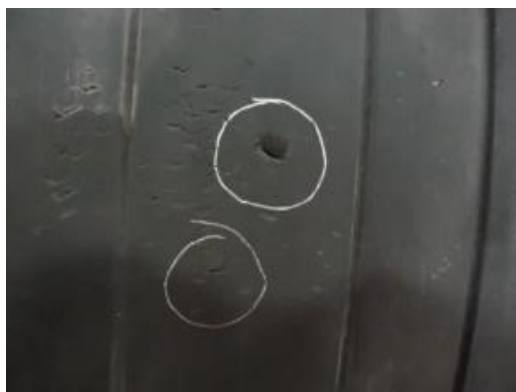
Figure 16. Cuts on wheel number 6 (paired with no. 5), produced on 30/01/2020
