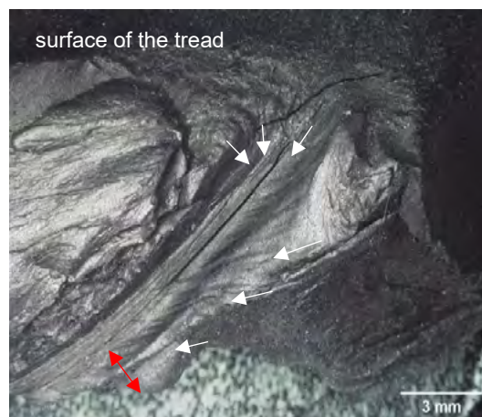
Figure 23. Deformation of the material in the tread of piece B
