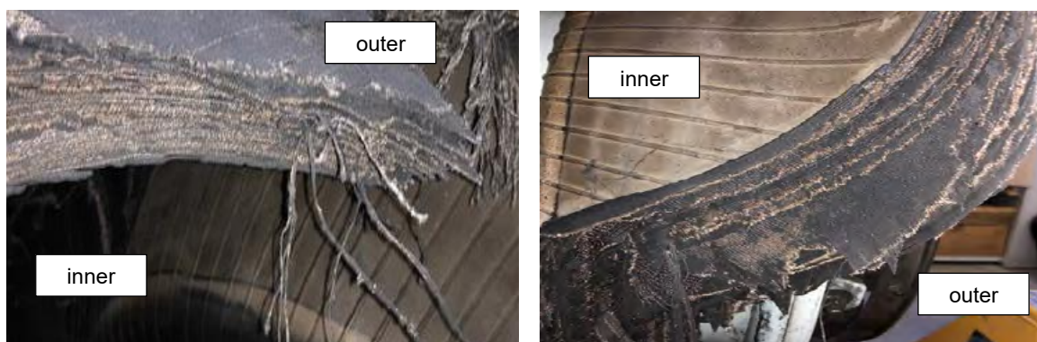
Figure 18. Direct ruptures (left) and tapered (right) in the casing of tyre no. 5
