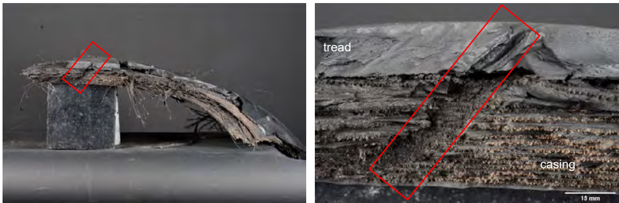
Figure 22. Perforation in piece B (casing and tread)
