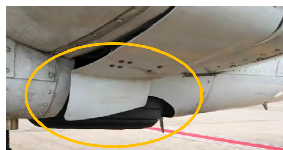
Photograph 18: Closed position of bent left MLG door
