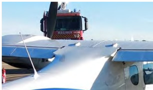
Photograph 3: Position of the flaps after the incident landing
