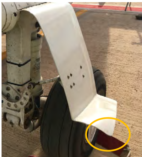
Photograph 15: Bent left MLG wheel well door
