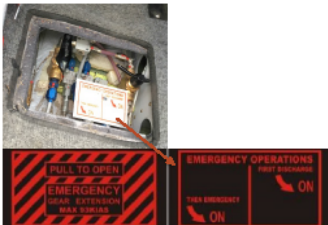
Photograph 24. Emergency gear extension panel
