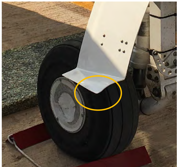
Photograph 16: Bent right MLG wheel well door
