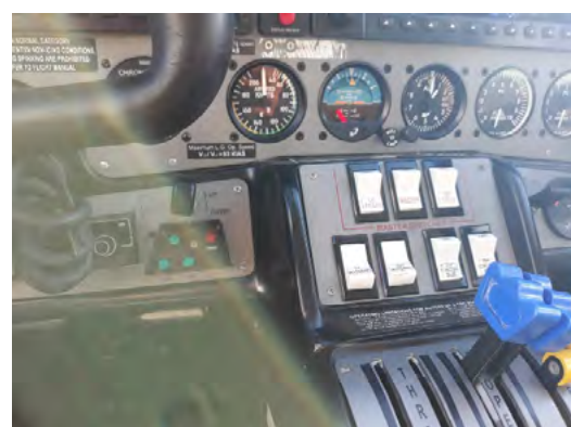
Photograph 5: Position of landing gear lever
