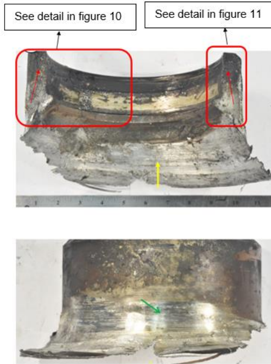
Figure 9 – Interior and exterior view of the largest of the inner wheel half hub fragments.
