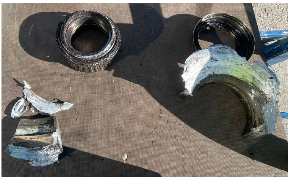
Figure 6 - Associated fractures to the affected wheel.
