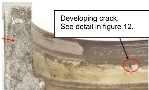
Figure 10 – Close-up of the inner wheel half hub fracture surface (1).
