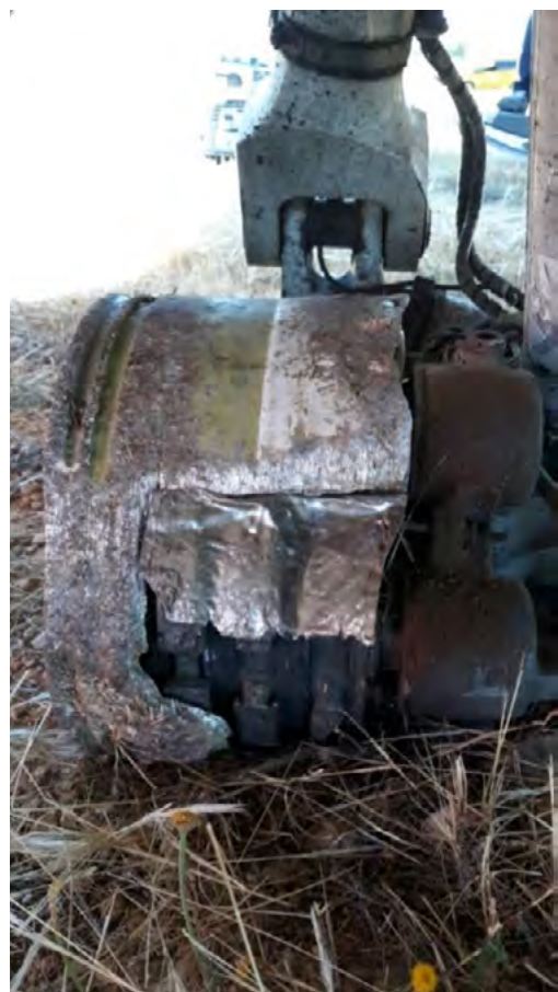
Photograph 8 right: MLG LH, wheel assembly
