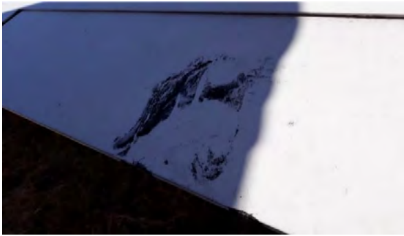
Photograph 11: LH Damage to inboard flap, top side
