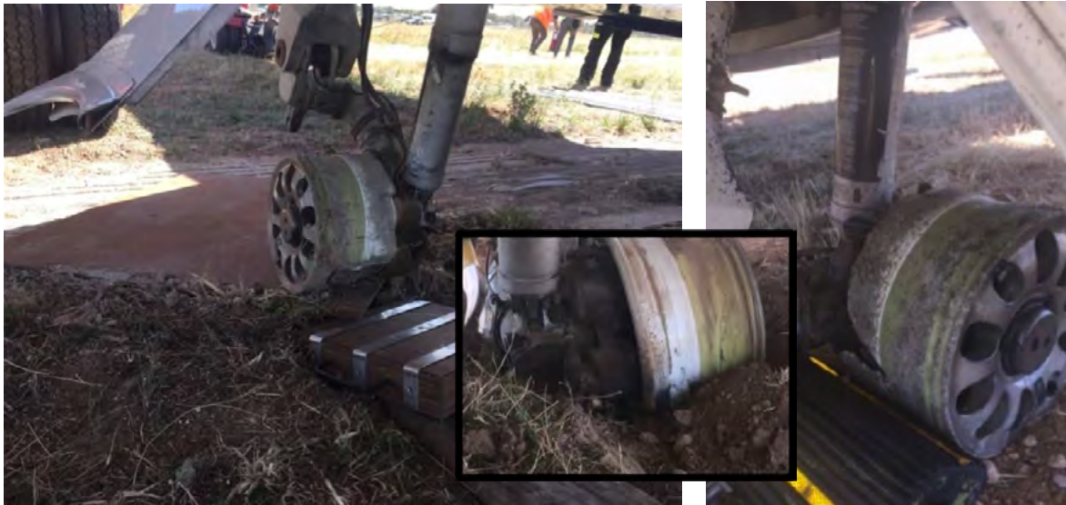
Photograph 9: MLG LH, rim, detail of the brake housing surfaces
