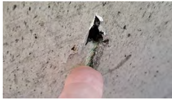
Photograph 12 and 13: LH Damage to inboard flap, underside and detail of puncture hole
