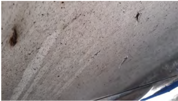
Photograph 12 and 13: LH Damage to inboard flap, underside and detail of puncture hole
