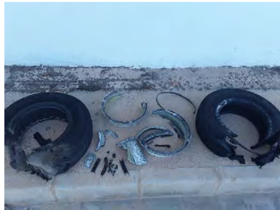
Photograph 23: Main landing gear tyres (to the right, LH wheel, to the left, RH wheel)
