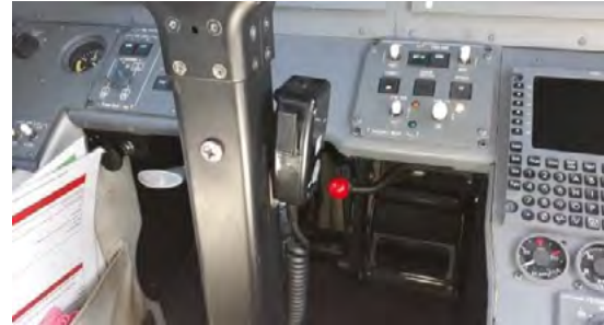
Photograph 19: Emergency brake lever
