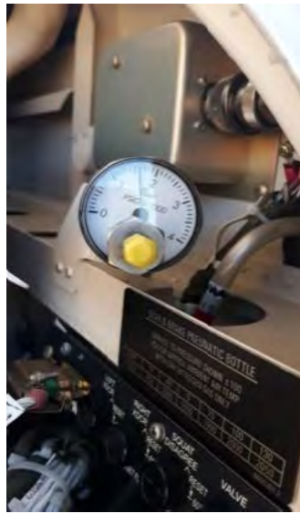
Left Photograph 15: Brake system accumulator
