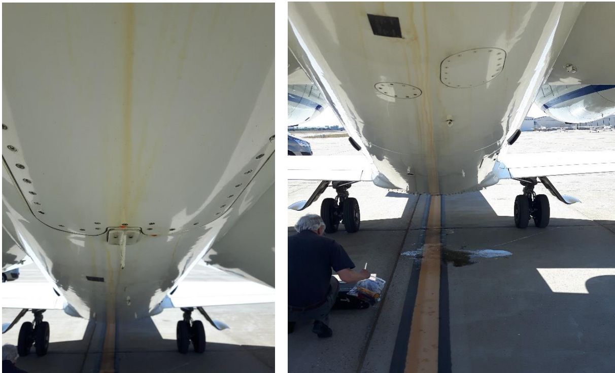
Photographs 4 and 5: Hydraulic fluid spills and stains on the fuselage
