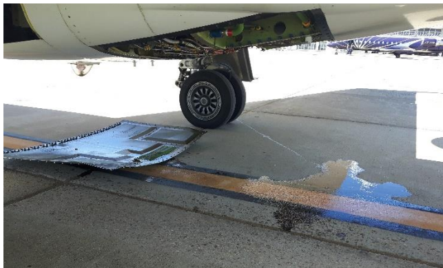
Photograph 2. Spilled hydraulic fluid
