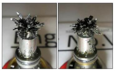
Figs. 15 & 16: Magnetic chip detectors MMCD and FBC MCD<sup>25</sup>
