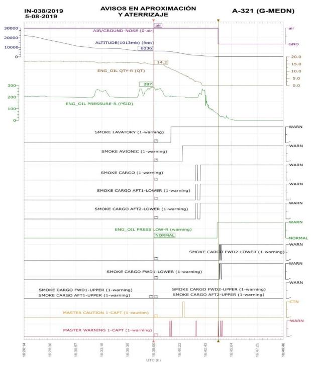
Fig. 12: Relevant parameters during the approach and landing phases
