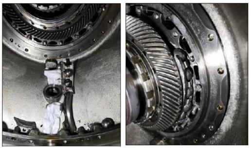
Figs. 19 & 20: Condition and remains of bearing no. 3 in situ
