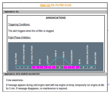
Fig. 23: Engine Oil Filter Clog procedure in the FCOM
