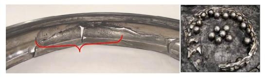
Figs. 17 & 18: Condition and remains of the cage and outer race of bearing no.3
