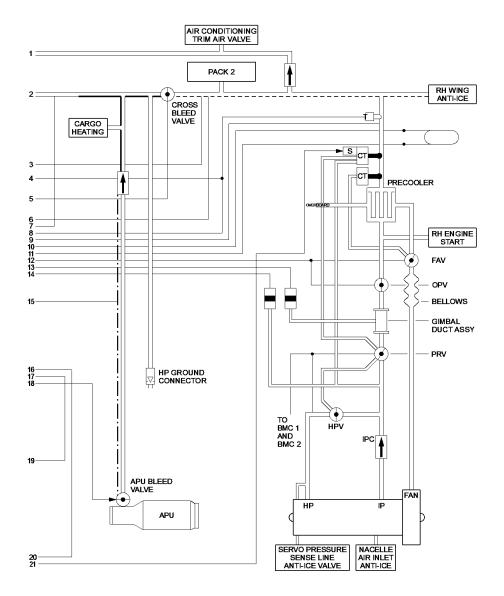
Fig. 5: Engine bleed air diagram
