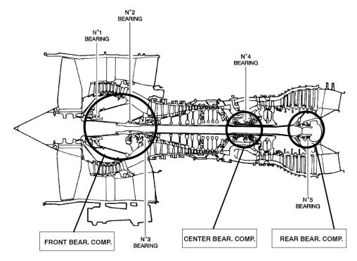
Fig. 2: Location of the bearings in the IAE V2500 engine
