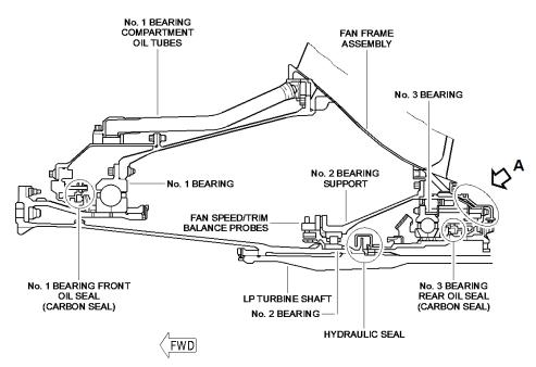
Fig. 4: Location of the seals in the front bearing compartment
