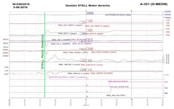
Fig. 11: Relevant parameters during the cruise phase in which the STALL occurred
