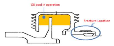
Fig. 21: Section of the hydraulic seal
