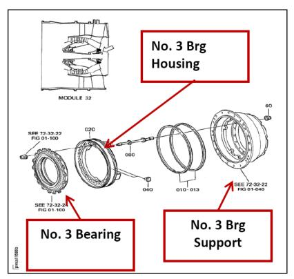
Bearing number 3 is a thrust bearing located in the Front Bearing Compartment (FBC).
