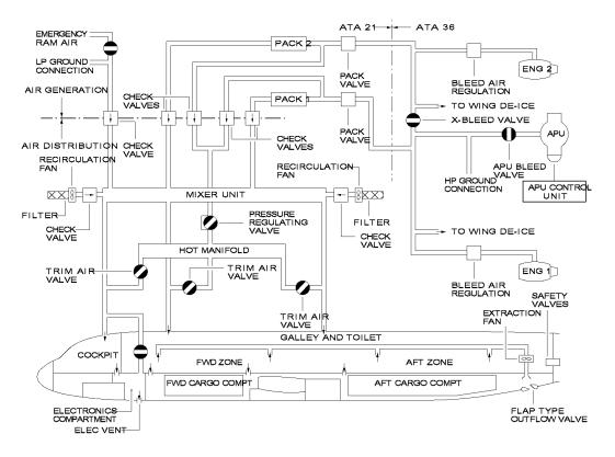
Fig. 6: Diagram of the air conditioning system
