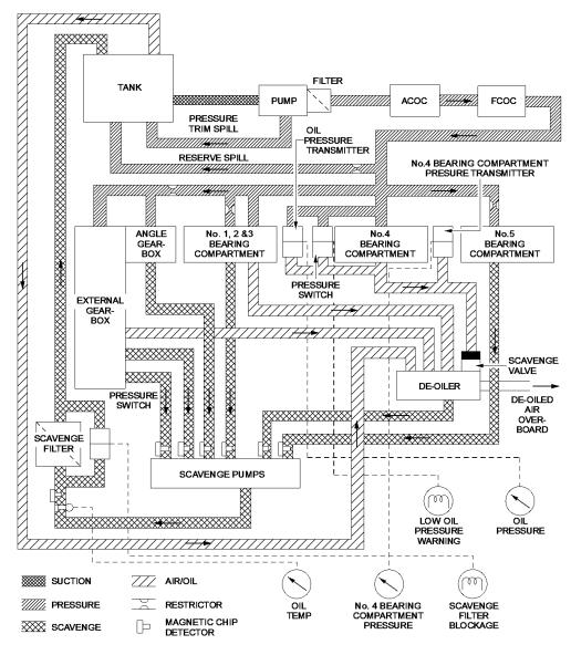
Fig. 7: Diagram of the engine oil system
