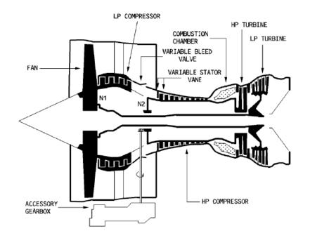
Fig. 1: IAE V2500 Engine diagram
