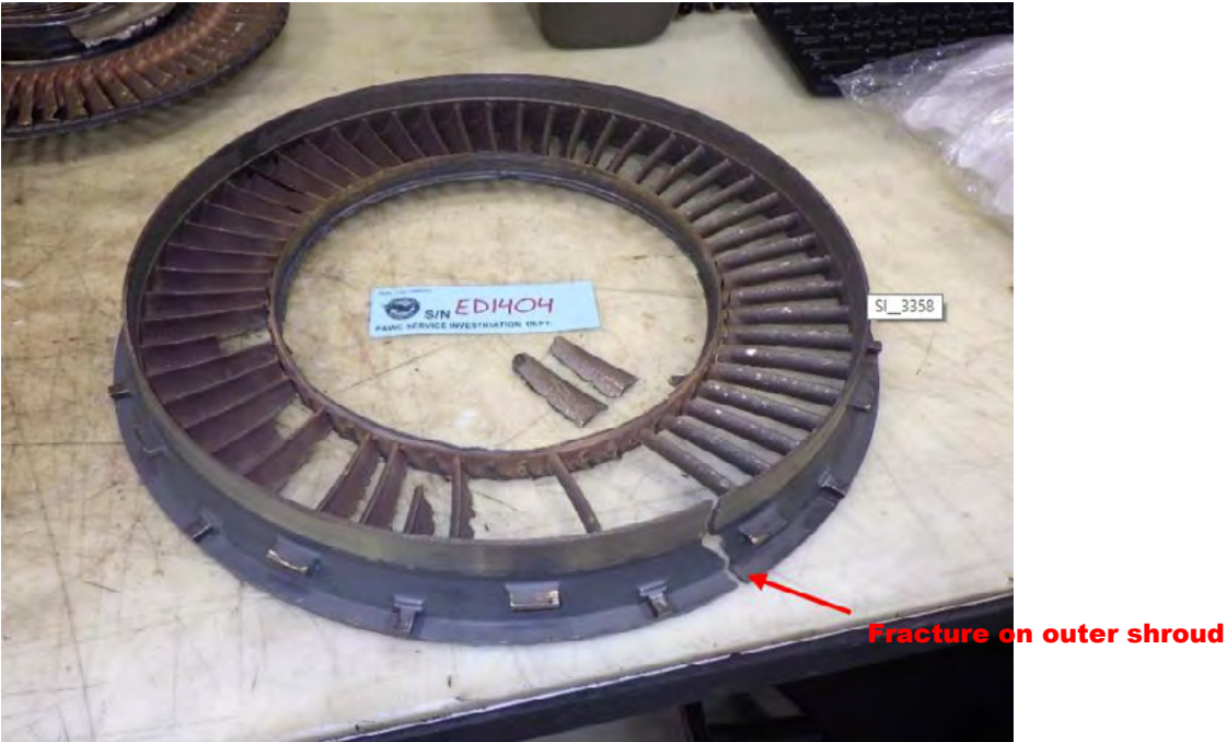
Figure 8. Damage to PT2 stator
