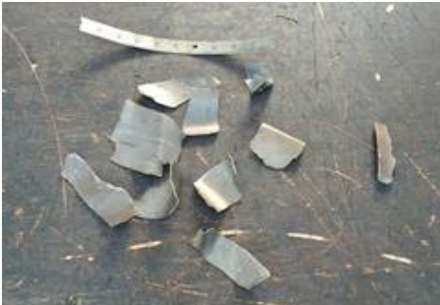
Figure 1. Fragments removed from the runway
