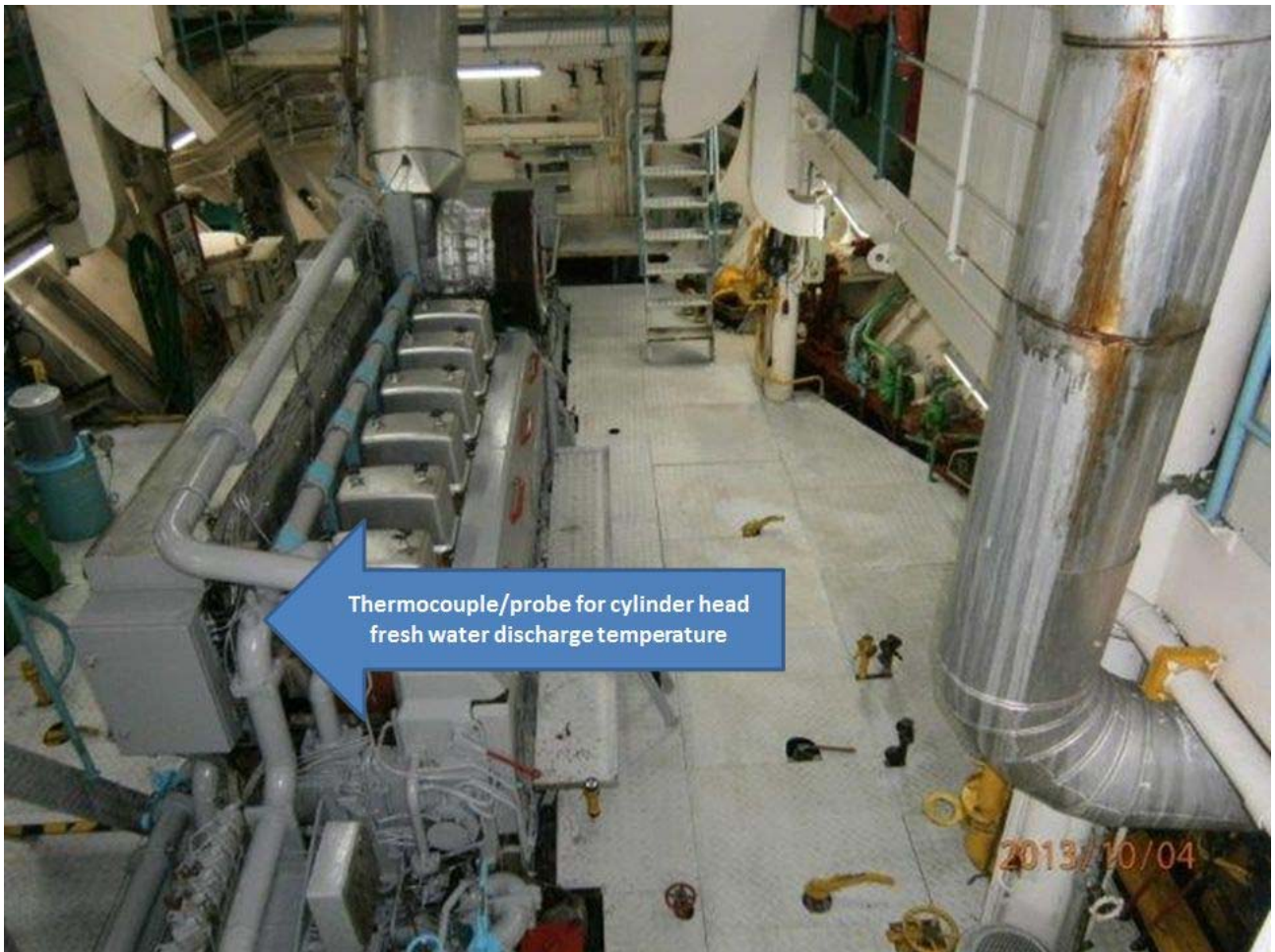
Figure 4. Location of the Sensor whose reading generated a High Temperature Alarm and subsequent Stop of Propulsion Engine Operation.
