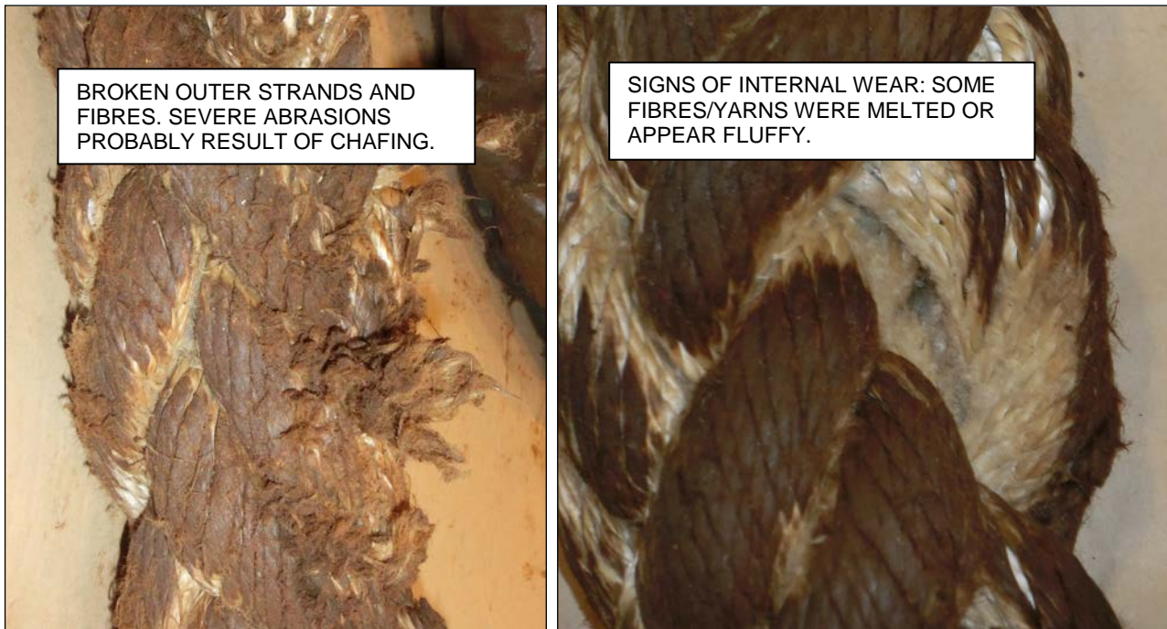
Figure 10: Details of parted rope. Both pictures show discolouration from grease Source: DMAIB
