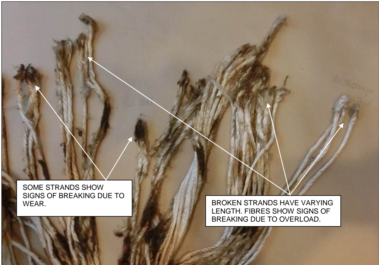
Figure 9: Details of the parted rope end Source: DMAIB
