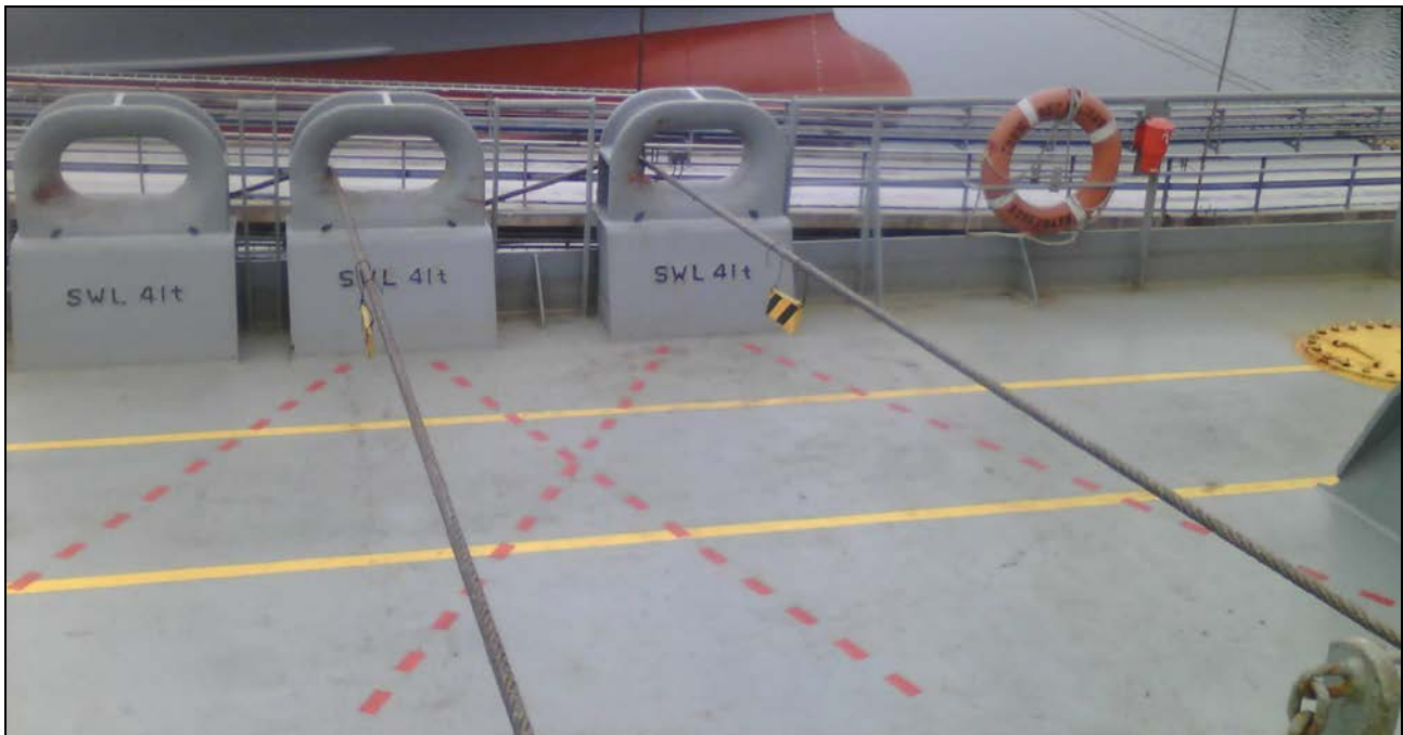
Figure 8: Snap back zones at starboard side forward, TORM REPUBLICAN Source: DMAIB
