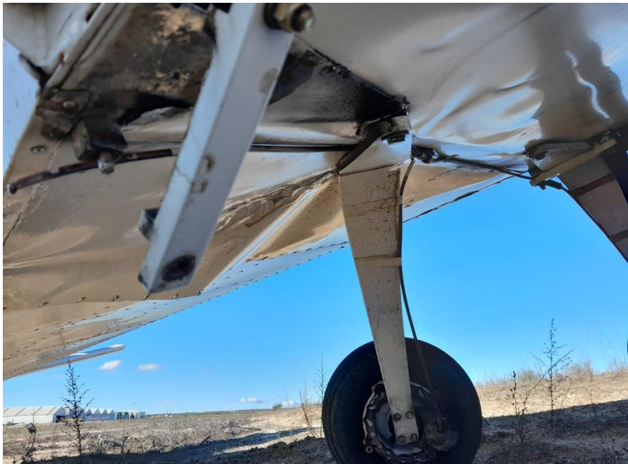
Fig. no. 9 - Close-up of the detachment of the right leaf spring
