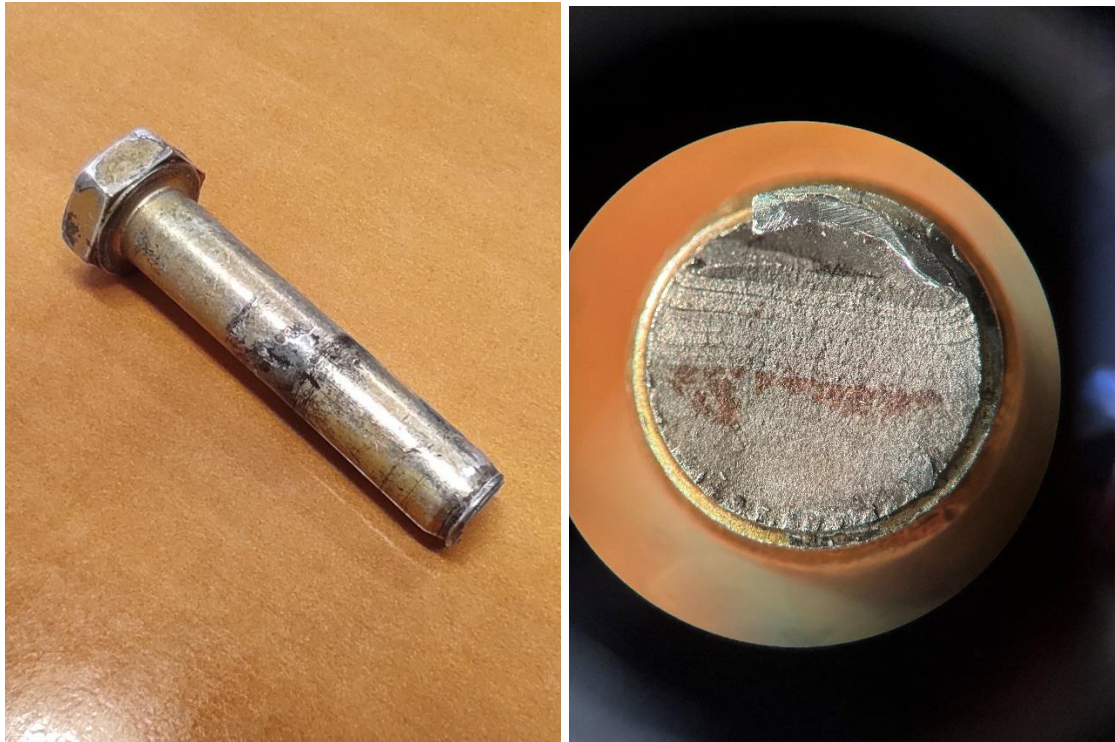
Fig. no. 11 - Close-up of the ruptured bolt
