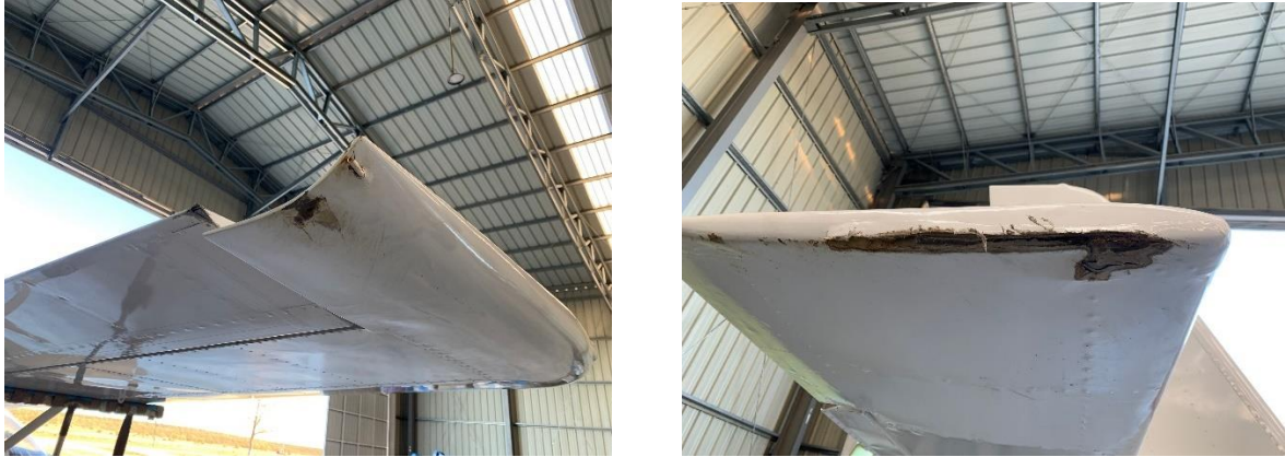
Fig. no. 10.- Damage to the wing and right stabiliser
