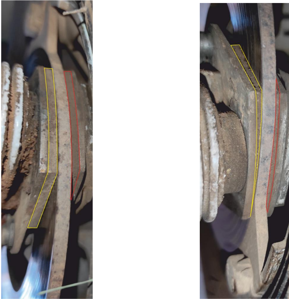
Fig. no. 5.- Condition of the brake pads
