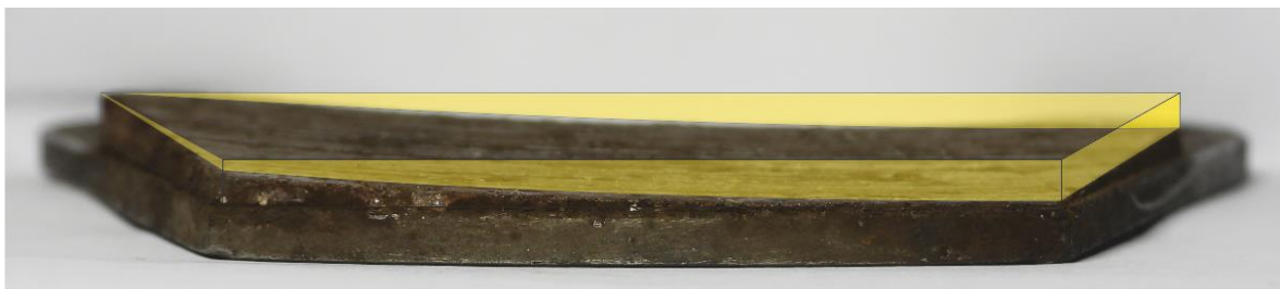
Fig. no. 4 - Wear to the right inner brake pad
