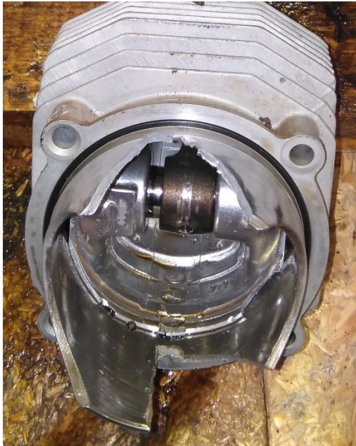
Figure 15: Close-up of breakages on cylinder sleeve and piston #2.
