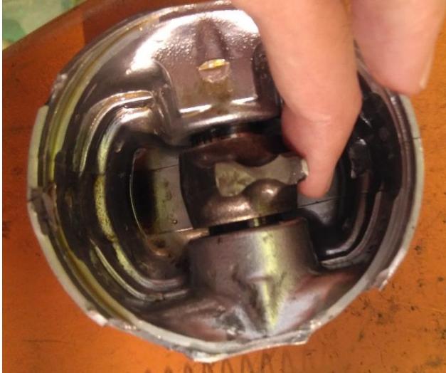
Figure 10: Close-up of connecting rod rupture (foot end).
