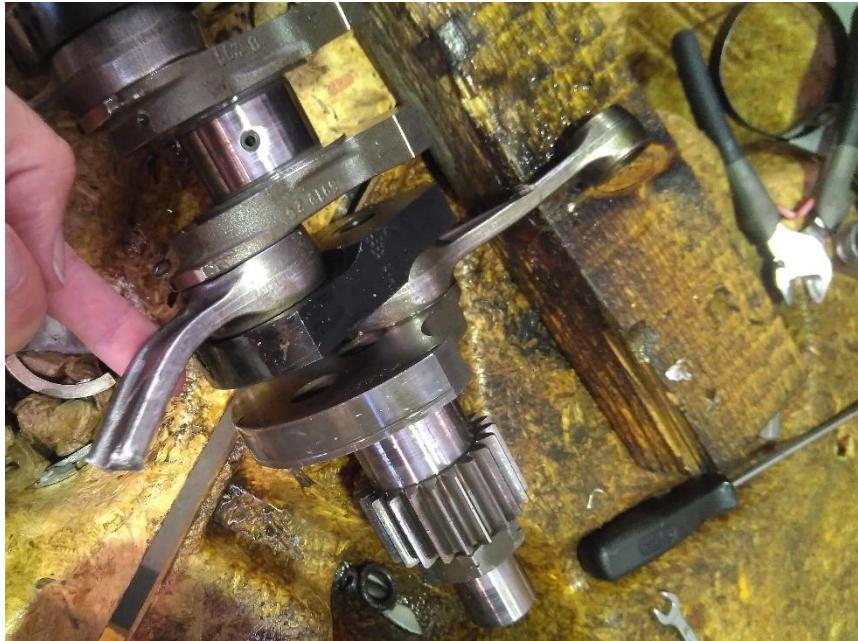
Figure 13: Connecting rod rupture (overview).
