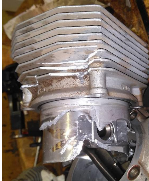
Figure 16: Close-up of breakages on cylinder sleeve and piston #1.
