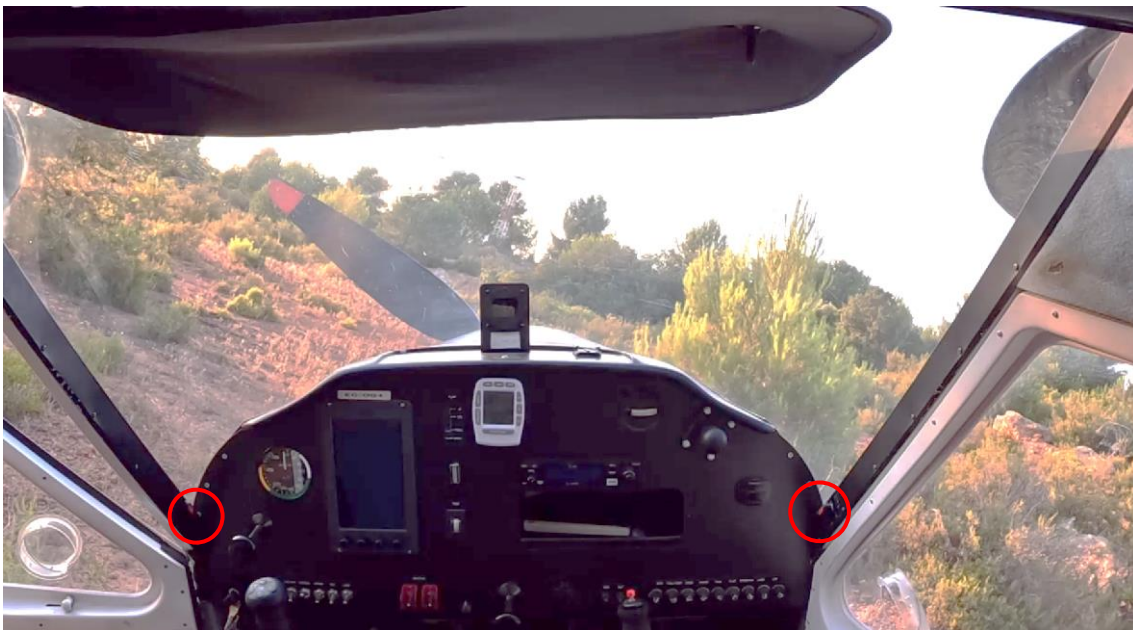
FIG. 1 POSITION OF FUEL VALVES AFTER THE ACCIDENT
