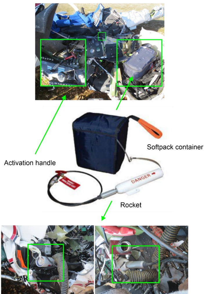
Figure 9 - Ballistic rescue parachute system components in the aircraft wreckage.
