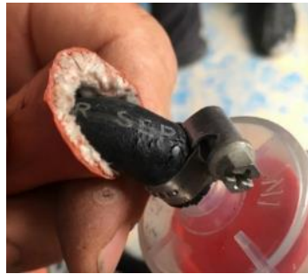
Photograph 18. Cracked fuel filter intake hose
