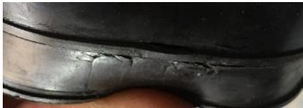
Photograph 17. Cracked intake hose
