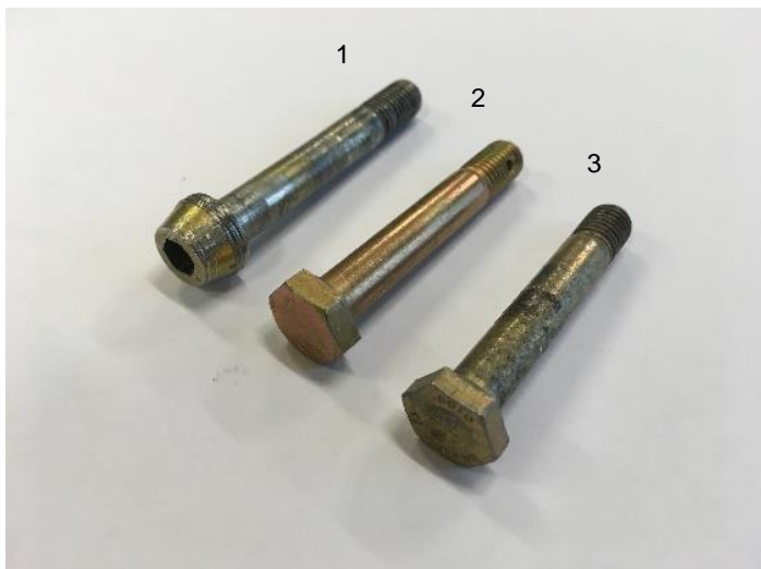
Photograph 15. Main landing gear leaf spring attachment bolts
