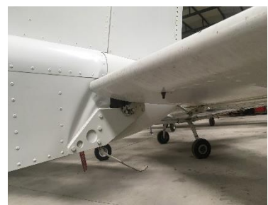
Photograph 12. Damage to the attachment of the left horizontal stabiliser
