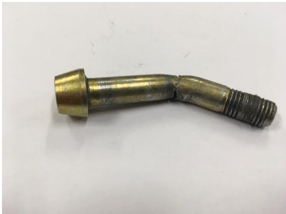
Photograph 18. Left leaf spring lateral bolt 1 after its removal from the incident aircraft
