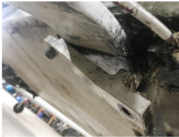
Photograph 7. Attachment of bracket to left leaf spring and fuselage
