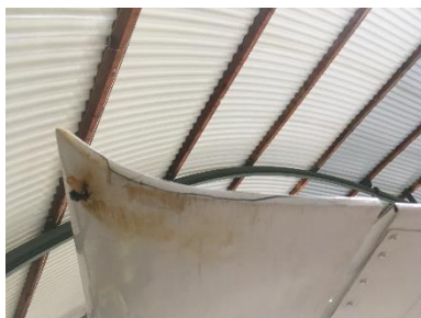
Photograph 10. Damage to underside of the left wing
