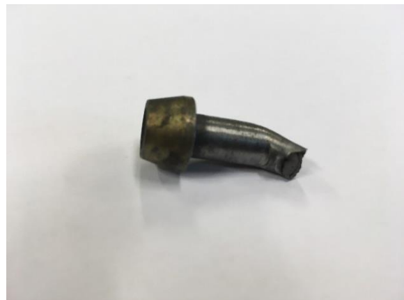
Photograph 19. Top half of severed lateral leaf spring bolt 2 after the incident
