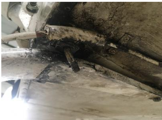
Photograph 8. Left leaf spring to fuselage lateral attachment bolt
