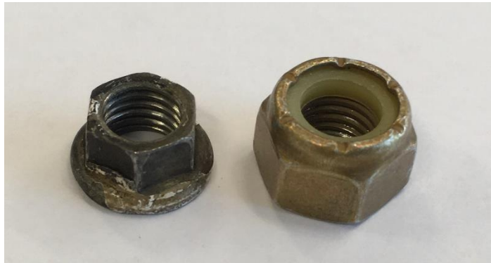
Photograph 14. Old self-locking nut used by the maintenance workshop involved in the incident and new nut used in the accident aircraft
