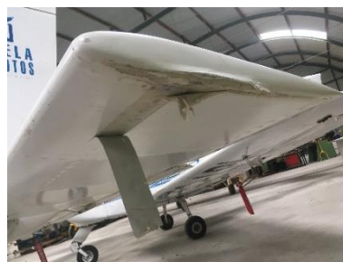
Photograph 11. Damage to the left underside of the horizontal stabiliser
