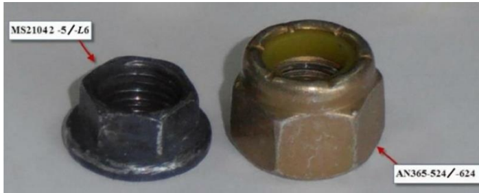
Photograph 13. Old and new self-locking nuts according to SB No.66
